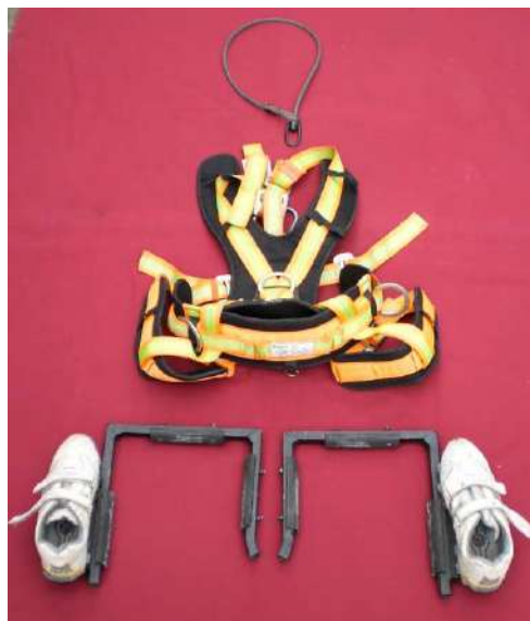
Safety attachment to the Joseph model of Paddle type coconut climbing device
