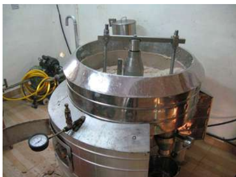
Fig. 13a Hot processing of VCO in VCO cooker (Biofuel based)
