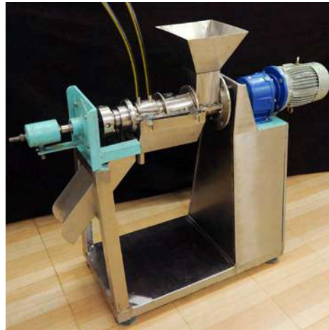
Fig. 11a Single screw milk expeller with cooling arrangement
