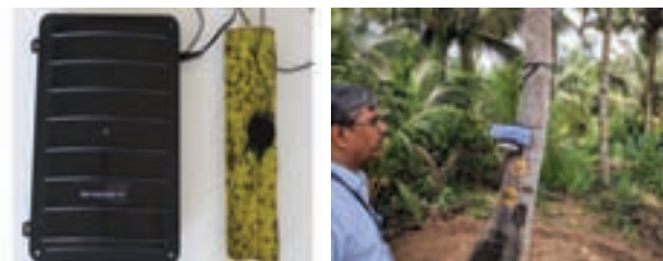
Fig. 5.3 Portable hardware in which the formulated algorithm was deployed to demonstrate the detection of grubs in the petiole and detection hardware set up in the field
