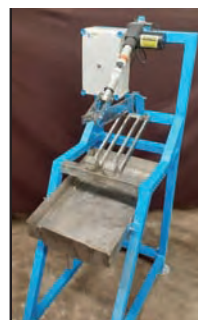
Fig. 40a. Semi-automatic tender coconut cutting machine
