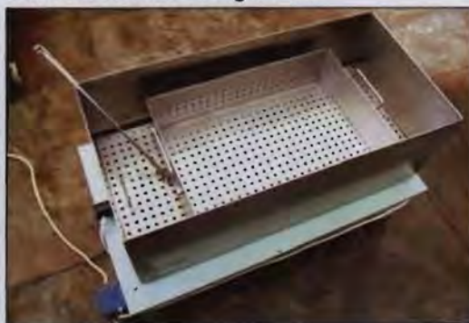
Fig. 9. Blanching unit for blanching of coconut slices
