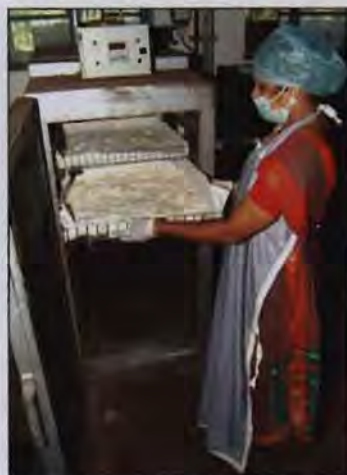
Fig. 10. Drying of coconut slices
