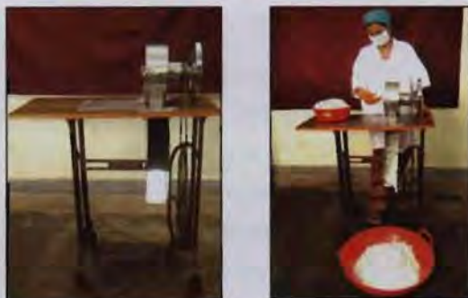
Fig. 8. Mechanical slicing of coconut kernel
