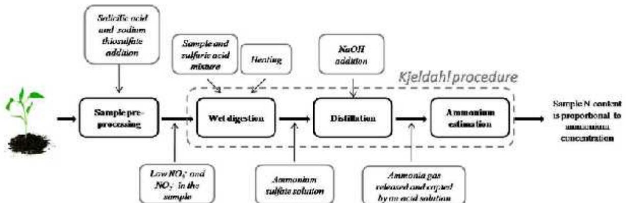
Working Principles: During digestion step all amino-N is converted to ammonical radical.
