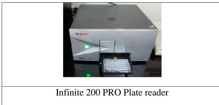
**Working principles:** Absorbance is a measure for the attenuation of monochromatic light when transmitted through a sample. If the sample contains only one species absorbing in that narrow band of wavelengths, the background corrected absorbance is proportional to the corresponding concentration of that species (Lambert-Beer's Law).
